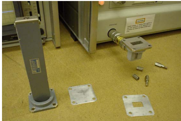
Figure 4.7 Coax to waveguide transition on the NA reflection test port.
