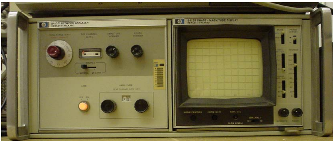
Figure 4.1(b) The HP8410 network analyzer with the HP8412 rectangular display (bench 2).
