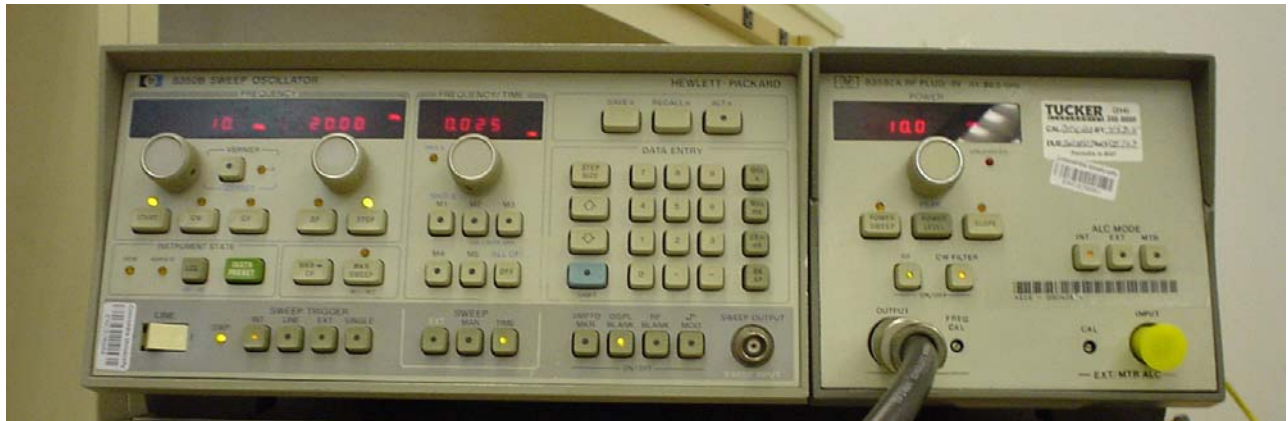
Figure 4.2 HP8350 sweeper with HP83592 plug-in unit for 0.1-20 GHz.
