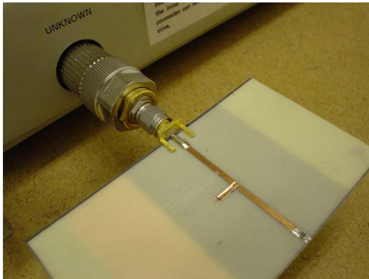
Figure 4.5 The stub tuner installed on the microstrip line, connected to the reflection port of the HP8743B transmission/reflection test set.
